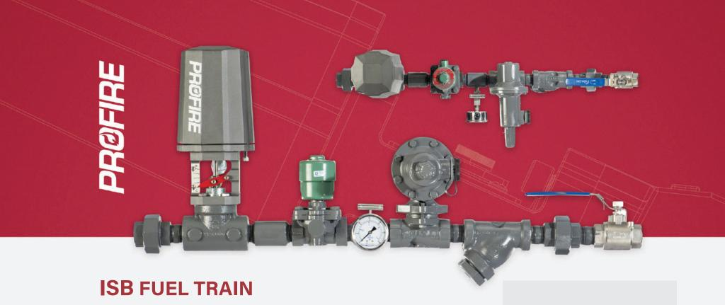
**ISB** is designed for applications using wet, low-quality fuel gas. To eliminate freezing pilot lines, regulators, solenoids and orifices, our Inline Pilotless design allows for safe ignition, soft start, and 4-20 mA temperature control. The Pilotless ISB fuel train features single-block main shutdown using an inline, gas-rated 6.5 C/I approved solenoid.
