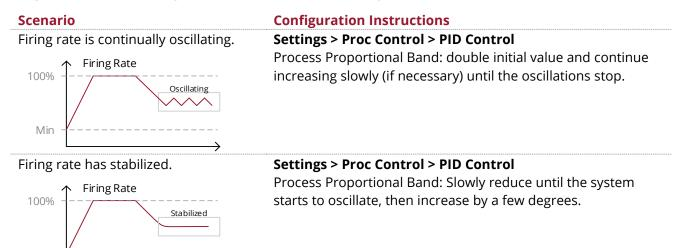
11. Test the **Proportional Band** setting - allow the process temperature to stabilize, then increase the **Process Setpoint** by 2 degrees to test the response of the system to a **Process Setpoint** change. Adjust settings as required in accordance with the following:
