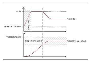
If the process is cold, the firing rate ramps up and holds at 100% until the process temperature reaches a temperature equal to the **Process Setpoint** minus the **Proportional Band**. At this point, the firing rate decreases proportionally as the temperature approaches the **Process Setpoint**. The firing rate settles between the configured TCV **Minimum Position** and 100%, and the process temperature settles below the configured **Process Setpoint**.
