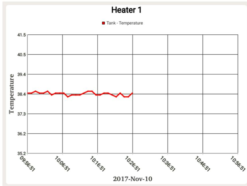
Use the +/- keys to size the graph. Ideally, the system should oscillate four times before stabilizing. If the process does not oscillate at all then the proportional band will need to be increased. If the process oscillates too much, then the proportional band should be decreased. A good rule for this process is to adjust the proportional band by roughly 20% each time.
