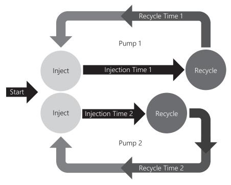
Figure 12 – Dual Pump Controller States
