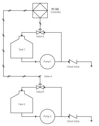
Figure 11 – Dual Pump Injection
