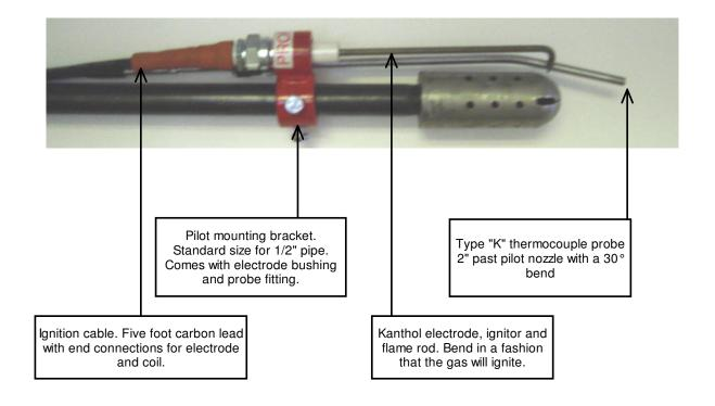
Pilot bracket assembly can be mounted on existing pilot. Brackets can be ordered to fit pilots 1/2" and up. Slip-stream applications are also acceptable, but may require custom length probe and ignition electrode.
