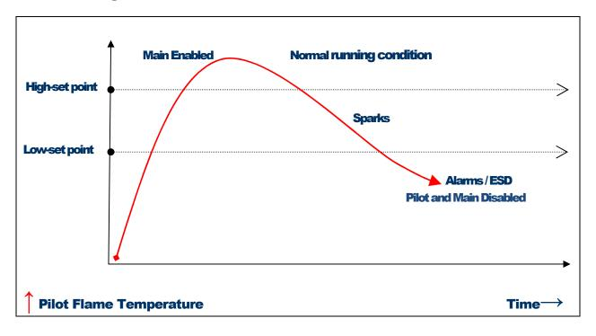
Type 'K' Thermocouple Output Chart
